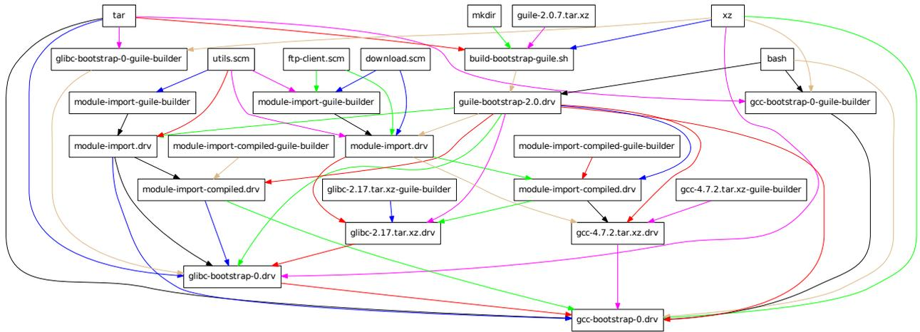
Figure 10: Dependency graph of the software distribution bootstrap.
