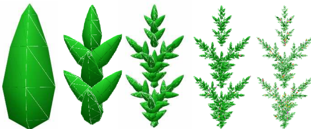
Figure 2. Series of iterations that generate a self-similar plant from an IFS consisting of 9 duplications of an initial object contracted by a factor 3 (theoretical fractal dimension D_T=2 ).
