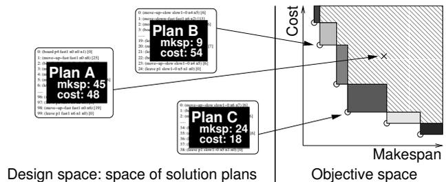
Figure 1: Design and objective spaces for a two-objectives planning problem. The hatched+grey area contains all images of possible solutions plans; this area defines the *hypervolume* of the set of circles, and the *hypervolume contribution* of each point is the grey area of the corresponding small rectangle (see Section 3). Circles are Pareto-optimal (non-dominated) solutions, aka the *Pareto front* of the problem at hand.
