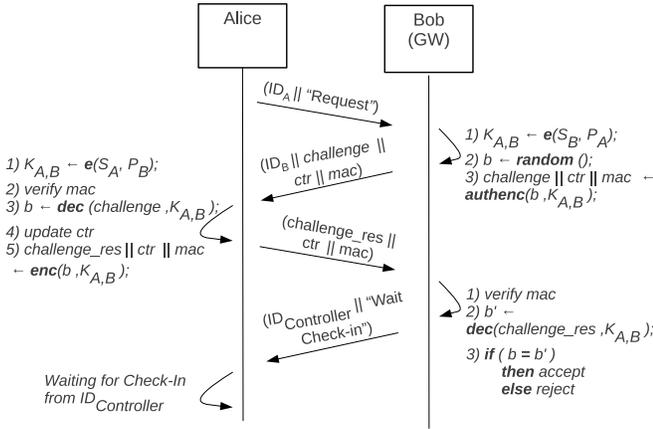
Fig. 3. Detailed handshaking procedure.
