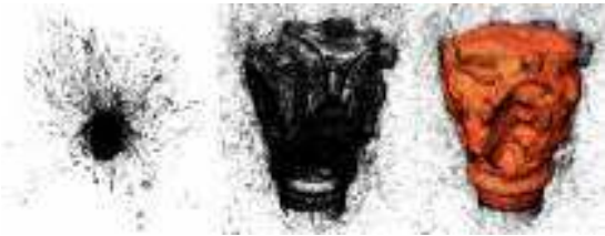
Figure 18: Noise and structured outliers. Left: raw point set. Middle: closeup on point set. Right: closeup on point set & reconstruction.
