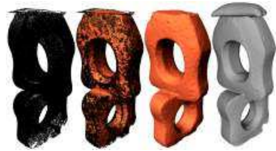
Figure 11: Low noise. From left to right: raw point set; point set & reconstruction; reconstruction only; Poisson reconstruction.
