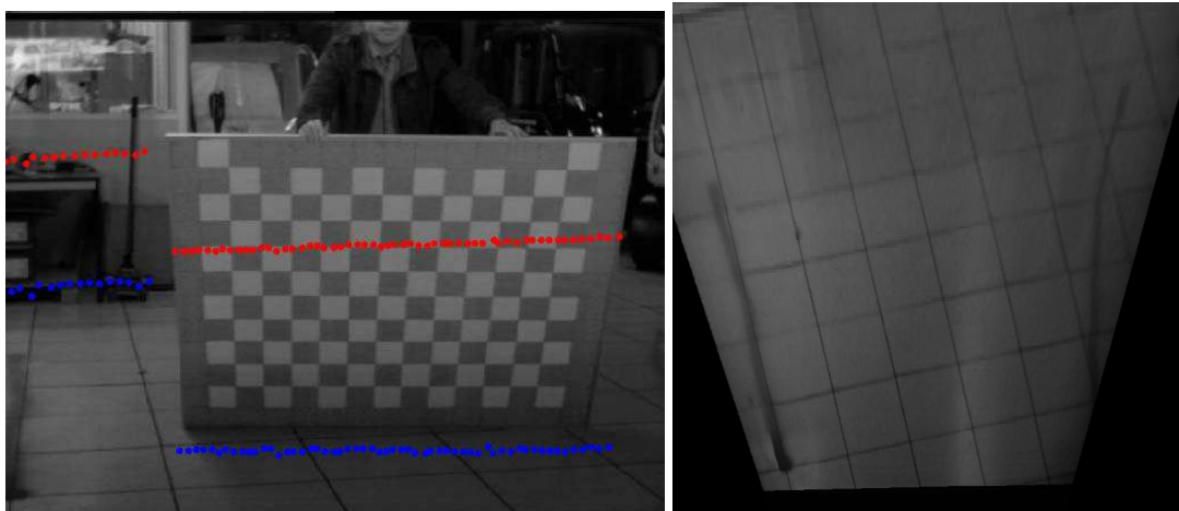
Fig.5. Intuitive effects: (Left) laser points and their ground projections; (Right) the bird-eye-view image of the garage floor
