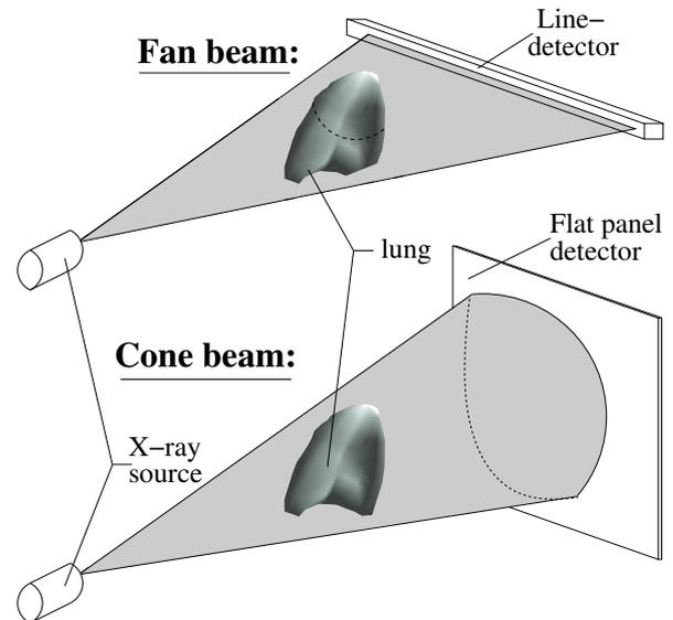
Figure 1: Tomography device: fan beam and cone beam
