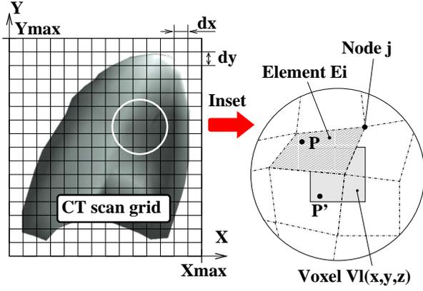
Figure 6: Geometrical parameter for CT scan convolution
