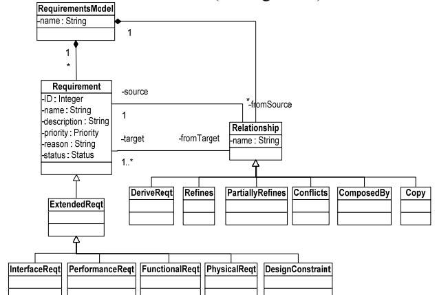
Figure 10 Specialized Requirements Metamodel for SysML Requirements
