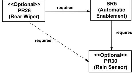
**Figure 15** Inferred relation in the Composed Models
