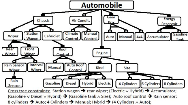
Figure 6 Product-line Model for the Automotive Example
