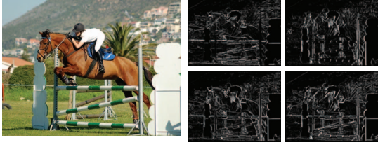
Figure 4. Left: Original image. Right: Edge-weighted gradient magnitude maps for four main orientations.
