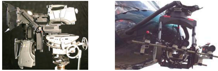
Figure 3.2: Examples of rigs: left, Binocle Brigger III in a studio configuration, a robotized rig for 3D TV, right, a heliborne rig with four cameras used by Binocle for the film La France entre ciel et mer
