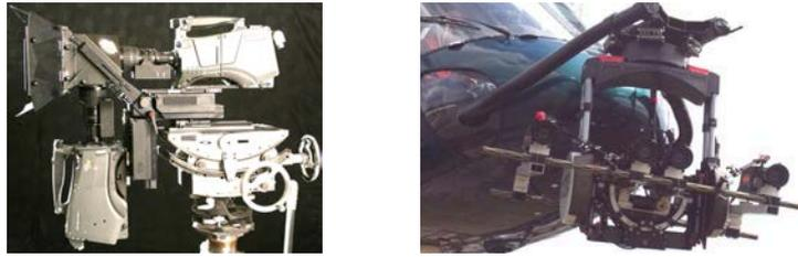
Figure 3.2: Examples of rigs: left, Binocle Brigger III in a studio configuration, a robotized rig for 3D TV, right, a heliborne rig with four cameras used by Binocle for the film *La France entre ciel et mer*
