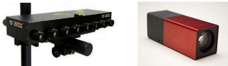
Figure 3.3: Examples of integrated cameras: left, a Cam-Box prototype camera with eight integrated perspectives developed by 3DTV Solutions and the University of Reims and, right, the Lytro plenoptic camera
