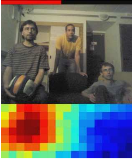
Fig. 5: People emitting sounds sequentially (top) and the corresponding aggregated statistic (5) for azimuth and elevation (bottom) roughly aligned with the image and when the leftmost person speaks. See the supplementary video for the entire sequence with the original sound track. Please notice the high level of noise in the signal due to fan inside the robot head.
