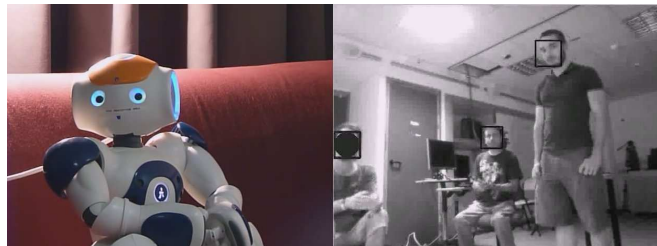
Fig. 1: The proposed method simultaneously detects and localizes an active speaker in an audio-visual scene. The humanoid robot NAO (left) turns its head towards the active speaker marked with a black disk (right). Please consult the supplementary video.
