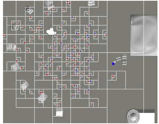
Figure 11: Using a quad-tree representation to reduce computational cost in querying characters in camera frustums and detecting events.
