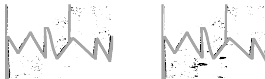
Figure 3. Bad pixels ( \delta = 1 ) using ENCC (left) and NCC (right) without sub-pixel refinement (Shaded area contains occlusions and depth discontinuities).
