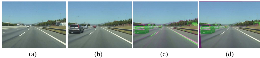
Fig. 4. (a) A query frame and (b) the best retrieved frame; (c) the space-time alignment after 2 and (d) after 10 iterations; differences between frames are indicated in lawn-green and hot-pink.
