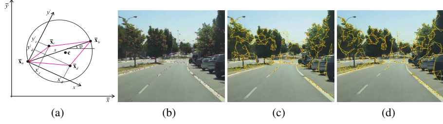
Fig. 2. (a) Geometric hashing using a quad structure; (b) query frame with extracted Harris points; (c) and (d) valid quads of the query and corresponding reference frame; red dots are quad centers.
