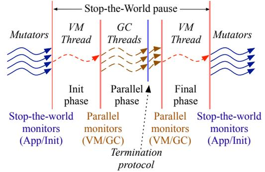
Figure 2. Phases of Parallel Scavenge
