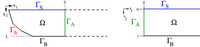
Figure 1: We look for a DtN on \Gamma_A . The solution on a semi-infinite rectangle is computed analytically.
