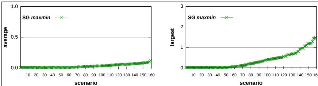
Fig. 3. Mean logarithmic error (left) and max logarithmic error (right) for all experimental scenarios for the flow-level model in [Velho and Legrand 2009], after removing *phase effects* by configuring GTNetS with the RED queue policy.
