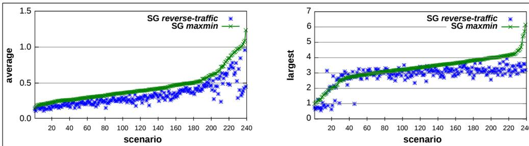
Fig. 11. Mean logarithmic error (left) and max logarithmic error (right) for all experimental scenarios for the flow-level model  $SG_{maxmin}$  in [Velho and Legrand 2009] and the improved reverse-traffic model  $SG_{reverse-traffic}$  proposed in Section 3.3, evaluated with topologies generated by Tiers.
