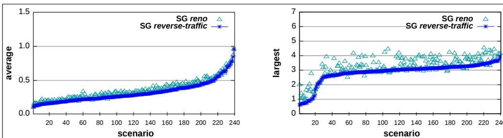
Fig. 12. Mean logarithmic error (left) and max logarithmic error (right) for all experimental scenarios for the reverse-traffic aware model based on Max-min,  $SG_{reverse-traffic}$ , and the arctan-based model in [Low 2003],  $SG_{reno}$ .
