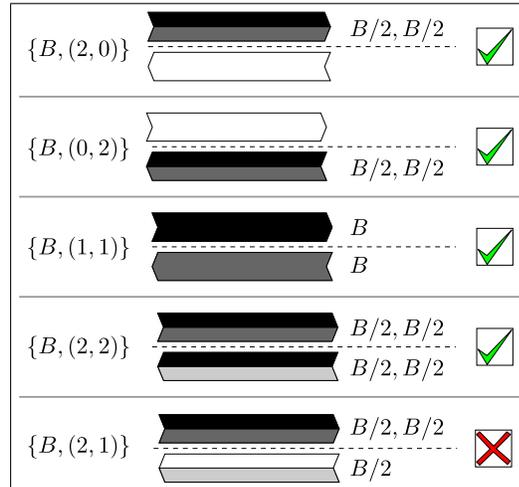
Fig. 8. Five reverse traffic interference scenarios:  $\{B, (n_1, n_2)\}$  denotes a scenario with one full-duplex link of capacity  $B$ , with  $n$  flows in one direction (shown above the dashed lines) and  $p$  flows in the reverse direction (shown below the dashed lines). The bandwidths allocated to the flows are shown on the right-hand side of each scenario. The last scenario shows an asymmetric situation.
