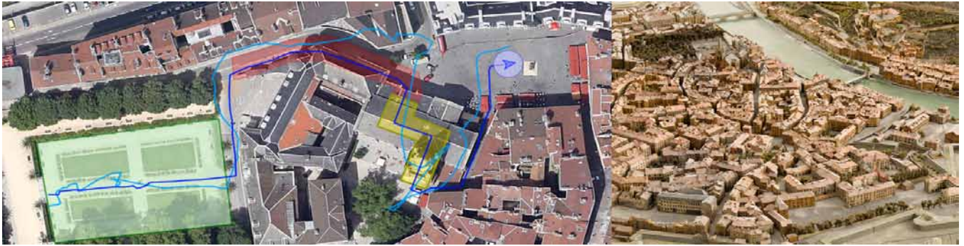
Figure 1: A route in dark blue where tracking was done using velocity-based DR . This route goes through a garden, a small street, a church and ends using a narrow street on an historical place of Grenoble (France) whose model (scale: 1/604) made of wood, paper, silk, metal and built from 1839 to 1848 is shown on the right. The corresponding GPS track is in light blue.
