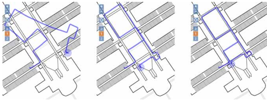
Figure 4: Navigation using only phone'sensors and based on dead-reckoning based is sensitive to gyroscope drift (left). With the help of a map, this drift can be corrected (center) as well as the distance computed using physiological models (right). The route shown is inside a public building and is passing through stairs to go from floor level 2 to floor level 1. No landmark validation was necessary to navigate in this building.
