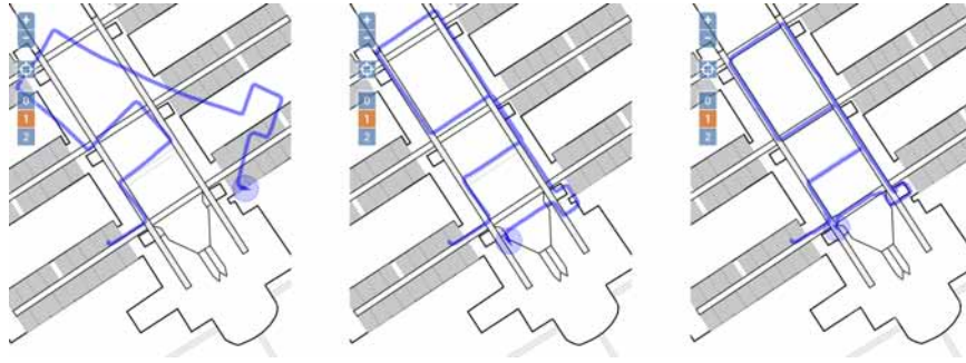
Figure 4: Navigation using only phone'sensors and based on dead-reckoning based is sensitive to gyroscope drift (left). With the help of a map, this drift can be corrected (center) as well as the distance computed using physiological models (right). The route shown is inside a public building and is passing through stairs to go from floor level 2 to floor level 1. No landmark validation was necessary to navigate in this building.
