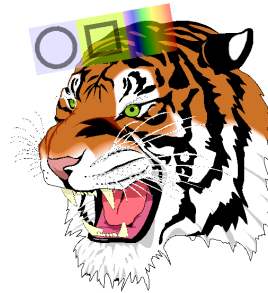
Figure 1: A rich SVG document, edited with a translucent toolglass. The tiger is rendered at 200 fps on a 1Ghz P3 + GeForce 2 GTS.
