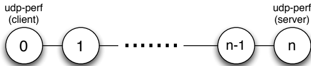
Figure 2: Experimental topology to estimate packet processing rate.
