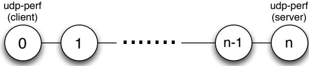
Figure 2: Experimental topology to estimate packet processing rate.
