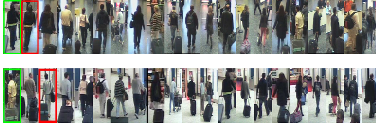
Fig. 3.6: Example of the person re-identification on i-LIDS-MA. The left-most image is the probe image. The remaining images are the top 20 matched gallery images. The red boxes highlight the correct matches.
