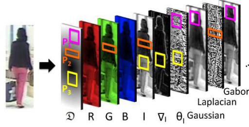
Fig. 3.4: A meta covariance feature space. Example of three different covariance features. Every covariance is extracted from a region ( P ), distance layer ( \mathcal{D} ) and three channel functions (e.g. bottom covariance feature is extracted from region P_3 using layers: \mathcal{D} , I -intensity, \nabla_I -gradient magnitude and \theta_I -gradient orientation).
