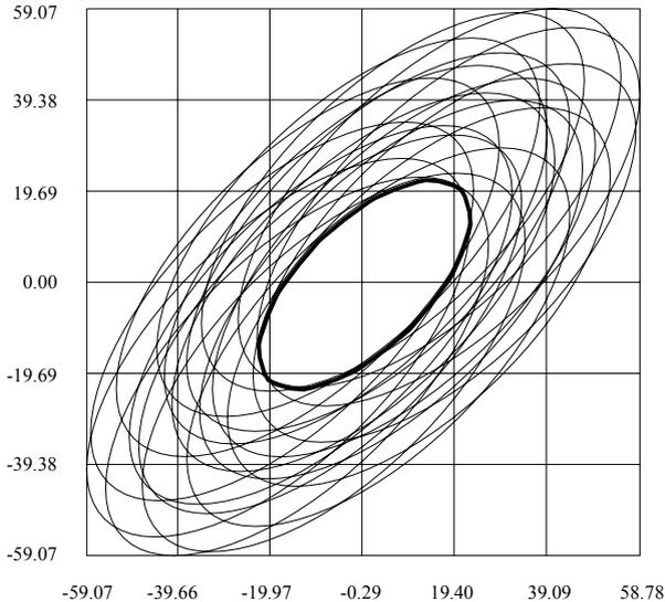
**Figure 1.1.** The  $x$ ,  $y$  axes of this graph represent the base and platform radii of a Gough platform, respectively. The region with the border in thick line represents all possible values of radii so that the robot workspace will include a set of pre-defined line segments trajectory.
