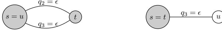
Fig. 3. Reduced graphs when applying RVR to the example of Figure 1, taking links in order \{s, u\}, \{s, t\} . Left: \mathcal{G}_1 ; right: \mathcal{G}_2 .
