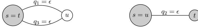
Fig. 2. Reduced graphs when applying RVR to the example of Figure 1, taking links in order \{s, t\}, \{s, u\} . Left: \mathcal{G}_1 ; right: \mathcal{G}_2 .
