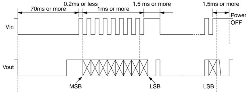
Fig. 2: The sensor timing diagram [Sharp Corporation 1997].
