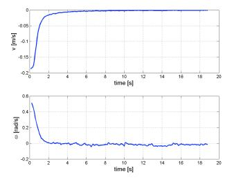
Fig. 19. Linear and angular velocity commands for the trajectory of Fig. 18
