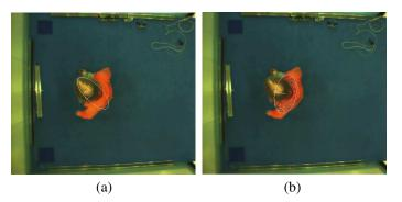
Fig. 16. Snapshots of the visual localization algorithm tracking a walking person; the elliptical model without head region (30) is used in (a), while the model with head region (31) is used in (b), resulting in a more accurate tracking
