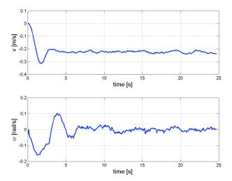
Fig. 21. Linear and angular velocity commands for the trajectory of Fig. 20
