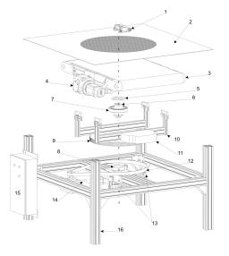
Fig. 12. Overview of the components of the *CyberCarpet* platform (referred to with  $\langle \rangle$  in the text)
