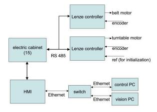
Fig. 14. Control and system drives architecture
