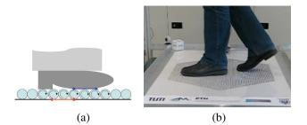
Fig. 1. The *CyberCarpet* platform: (a) the motion transmission principle; (b) the final small-scale realization
