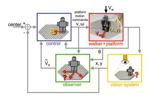
Fig. 2. Control system architecture of the CyberCarpet
