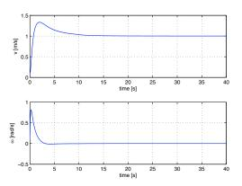
Fig. 5. Linear and angular velocity commands for the trajectory of Fig. 4
