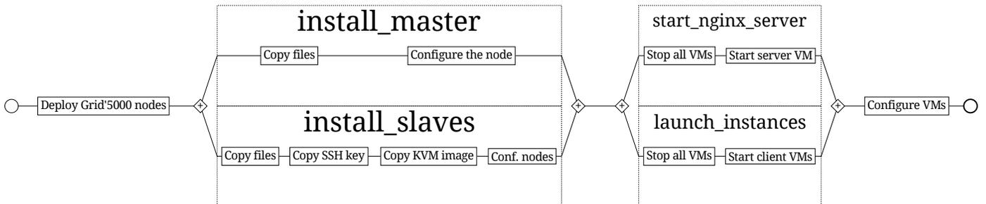
Figure 6. A full listing of workflows used to deploy a cloud-like testbed and an autogenerated graphical representation of the `deploy_cloud` workflow (thanks to the annotations inside comments). The blocks defined with `process` keyword describe workflows, whereas a block defined with `activity` contains a low-level Ruby code. Various patterns discussed in the paper are presented: failure handling, checkpoints, parallel execution and composable experiments.
