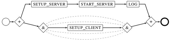
Figure 1. An example of a mapping between DSL and a workflow. Different language-level constructs (*parallel*, *forall*, *sequence*) result in respective workflow patterns (parallel execution of subworkflows, a parallel loop and sequential execution of activities). The workflow notation is based on Business Process Model and Notation (BPMN) with some extensions (the “ampersand notation” for a parallel loop, for example).
