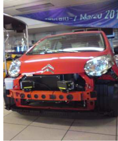
Figure 1. Automated vehicle developed at INRIA equipped with two laser rangefinders
