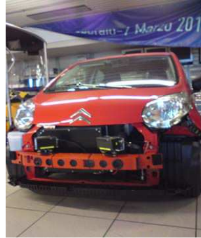
Figure 1. Automated vehicle developed at INRIA equipped with two laser rangefinders
