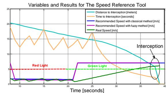
Figure 10 – Speed reference tool performance for the intersection problem in short distance
