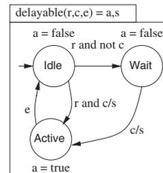
**Figure 3 Delayable task in textual and graphical syntax.** Figure 3 shows an example of a program with the BZR programming language. In the left hand side, we show the syntax of the language. In the right hand side, we depict the corresponding automaton.
