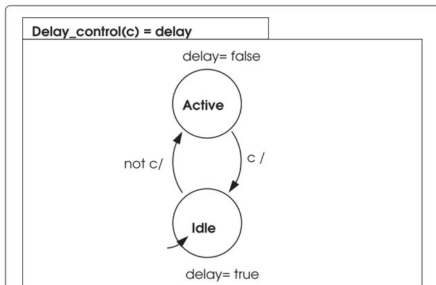
**Figure 6 Modelling the control of self-sizing.** Figure 6 models the control of the self-sizing adding operations.
