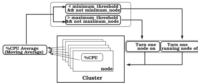
**Figure 1 Self-sizing manager.** Figure 1 shows the execution scheme of the server provisioning manager. The CPU utilization of the machines hosting the replicated servers are measured and a moving average is computed. If this moving average is higher than the fixed maximum threshold, the manager adds a new server on one unused machine. If the moving average is less than the fixed minimum threshold, the manager removes a server and turns the machine running the stopped server off.
