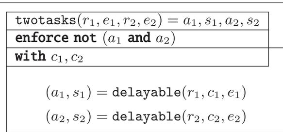
**Figure 4 Mutual exclusion enforced by DCS in BZR.** Figure 4 shows the design of a controller in BZR programming language. In this example we compose two instances of the program shown in Figure 3 and enforce a mutual exclusion between two instances.
