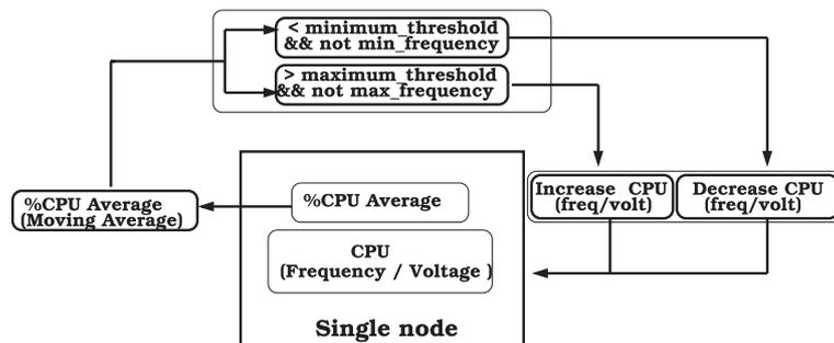
**Figure 2 Dvfs Manager.** Figure 2 shows the execution scheme of this manager. The CPU utilization of the machine is measured. If the CPU utilization is higher than the fixed maximum threshold, the manager increases the CPU frequency of the machine. If the CPU utilization is less than the fixed minimum threshold, the manager decreases the CPU frequency of the machine.
