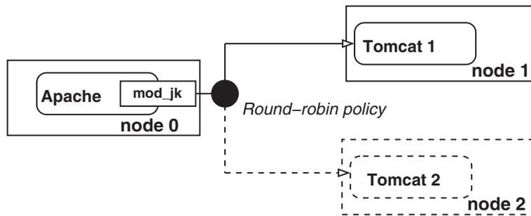
**Figure 10 Experimental Platform Architecture: Managed system.** Figure 10 shows the architecture of the managed system. It is a replicated-based system with replicated Tomcat servers and an Apache server acting as a load balancer.
