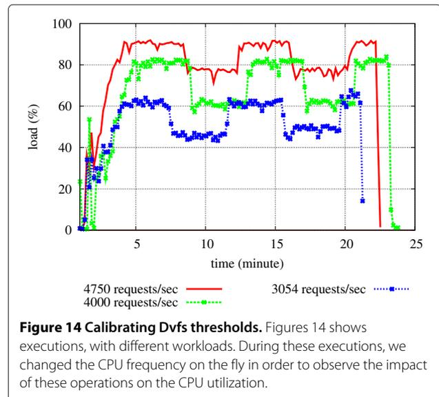
**Figure 14 Calibrating Dvfs thresholds.** Figures 14 shows executions, with different workloads. During these executions, we changed the CPU frequency on the fly in order to observe the impact of these operations on the CPU utilization.
