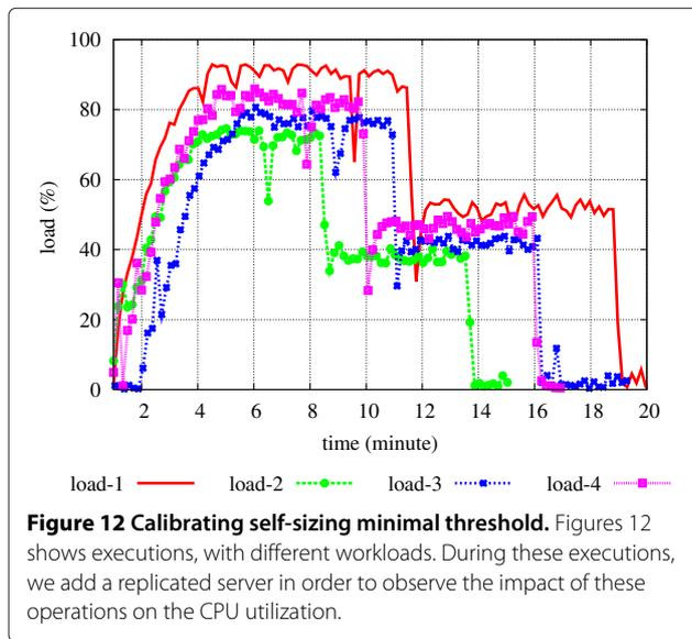
**Figure 12 Calibrating self-sizing minimal threshold.** Figures 12 shows executions, with different workloads. During these executions, we add a replicated server in order to observe the impact of these operations on the CPU utilization.
