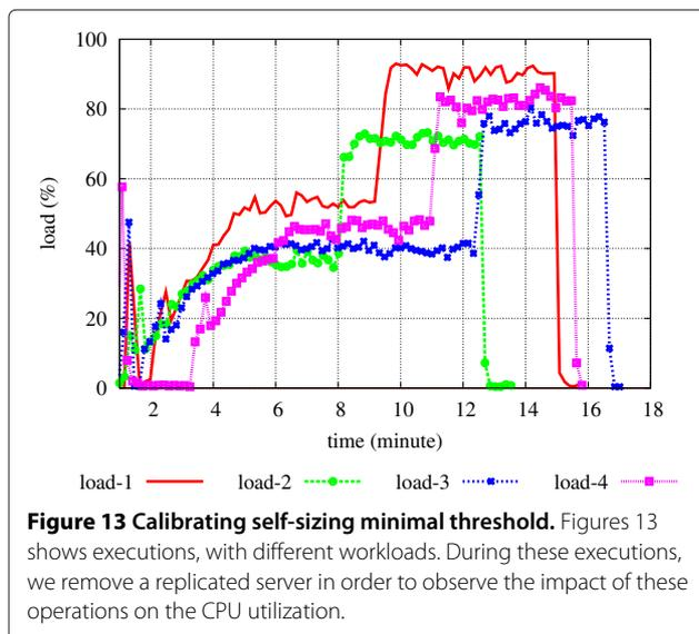
**Figure 13 Calibrating self-sizing minimal threshold.** Figures 13 shows executions, with different workloads. During these executions, we remove a replicated server in order to observe the impact of these operations on the CPU utilization.
