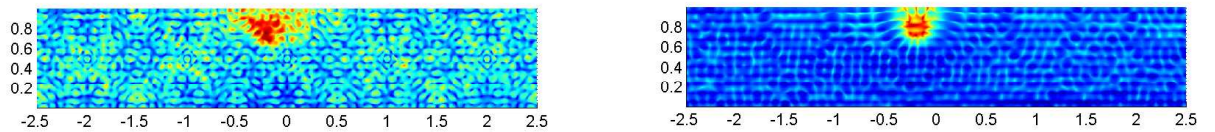
Figure 9. Amplitude of noise: 1%. Left: periodic waveguide. Right: homogeneous waveguide
