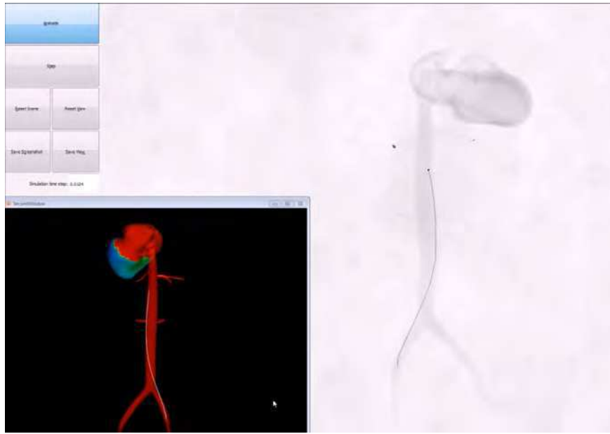
Figure 6: Catheter endovascular navigation in the simulator.
