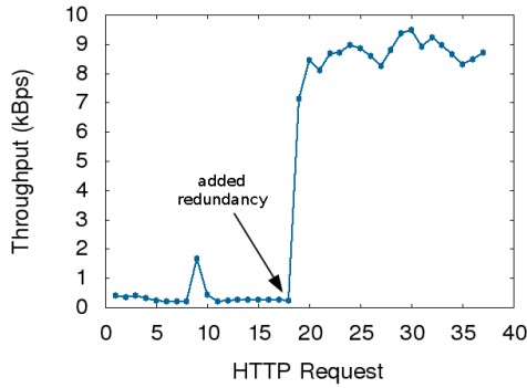
Figure 13: Throughput before and after the event of activating a redundant gateway with no QoS enforcement policy.
