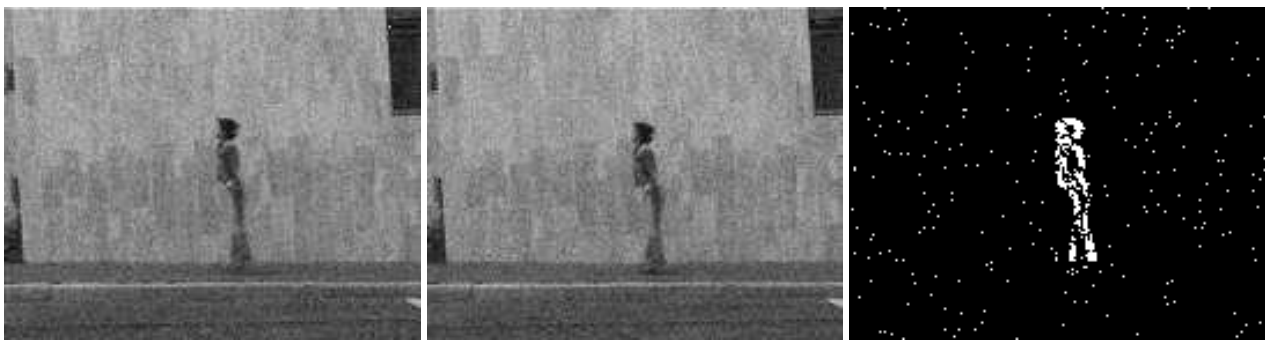
Figure 7. Two consecutive images ( 180 \times 144 ) perturbed by a Gaussian noise (standard deviation equal to 10), and the corresponding thresholded difference image.
