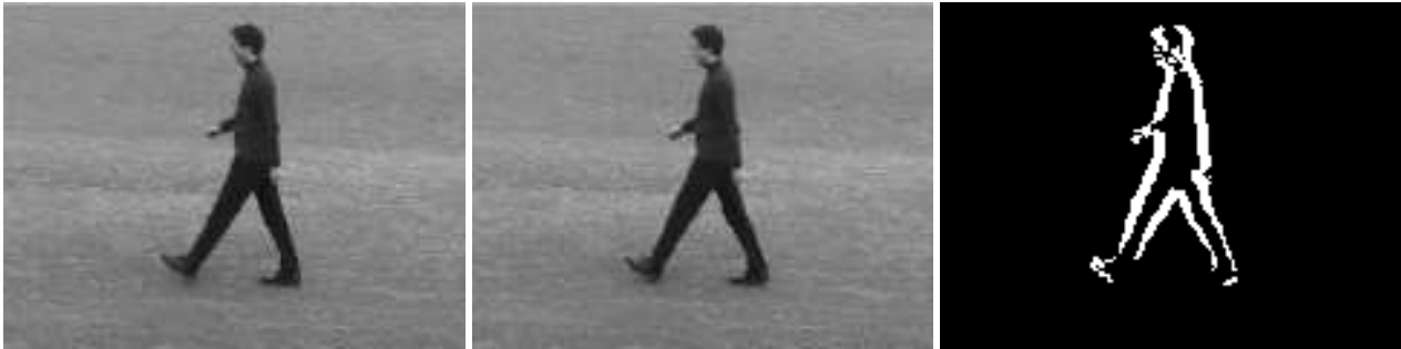
Figure 3. Two consecutive images ( 180 \times 144 ) taken from an image sequence, and the corresponding thresholded difference image.
