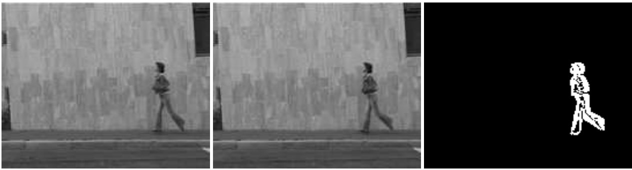
Figure 3. Two consecutive images ( 180 \times 144 ) taken from an image sequence, and the corresponding thresholded difference image.
