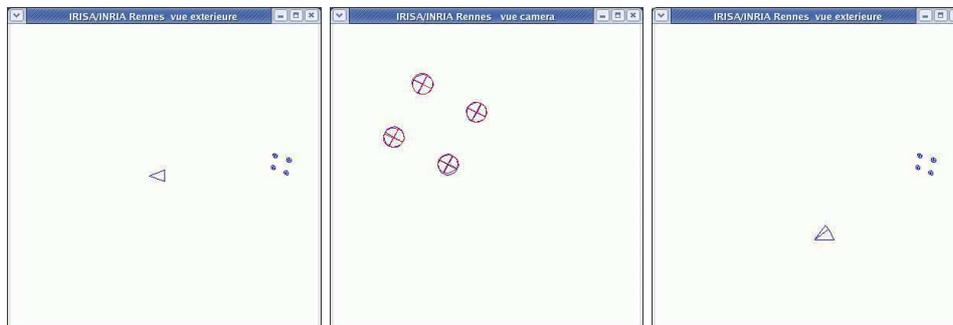
Figure 24.11: Two different camera poses (left and right) that provide almost the same image of four coplanar points (middle)
