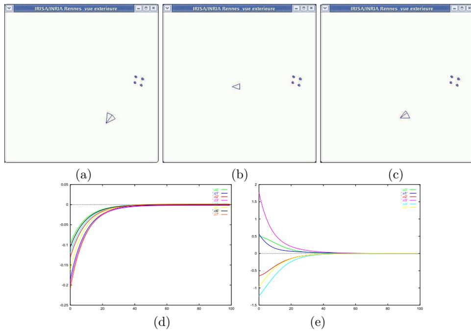
Figure 24.6: Reaching a local minimum using  $\mathbf{s} = (x_1, y_1, \dots, x_4, y_4)$  and  $\widehat{\mathbf{L}}_e^+ = \mathbf{L}_e^+$ : (a) initial configuration, (b) desired one, (c) configuration reached after the convergence of the control scheme, (d) evolution of the error  $\mathbf{e}$  at each iteration of the control scheme, (f) evolution of the six components of the camera velocity  $\mathbf{v}_c$ .
