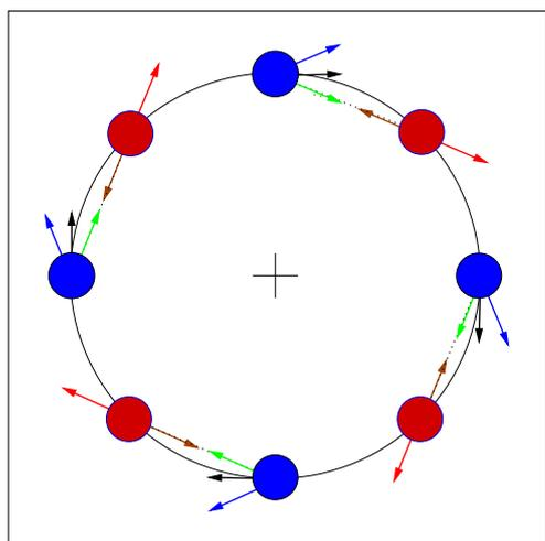
Figure 24.5: Geometrical interpretation of IBVS: going from the blue position to the red one. In red, image motion when  $\mathbf{L}_{\mathbf{e}}^+$  is used in the control scheme; in blue, when  $\mathbf{L}_{\mathbf{e}^*}^+$  is used; and in black when  $(\mathbf{L}_{\mathbf{e}}/2 + \mathbf{L}_{\mathbf{e}^*}/2)^+$  is used (see text more more details).
