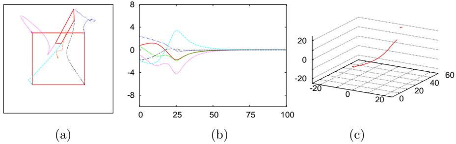
Figure 24.2: System behavior using  $\mathbf{s} = (x_1, y_1, \dots, x_4, y_4)$  and  $\widehat{\mathbf{L}}_{\mathbf{e}^*}^+ = \mathbf{L}_{\mathbf{e}^*}^+$ : (a) image points trajectories including the trajectory of the center of the square which is not used in the control scheme, (b)  $\mathbf{v}_c$  components (cm/s and dg/s) computed at each iteration of the control scheme, (c) 3D trajectory of the camera optical center expressed in  $\mathcal{R}_{c^*}$  (cm).
