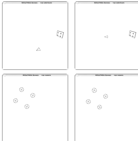
Figure 6.6. Example of two distinct positions of the camera with respect to the object (top) that provide similar images of this object (bottom)
