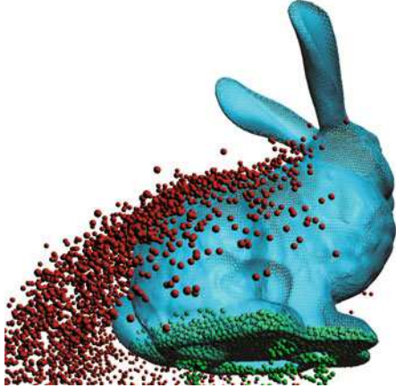
Figure 3 A scene demonstrating collisions with both sides of a mesh and support for non-closed meshes. The green particles were created inside the Bunny model and are interacting with the backside of the mesh surface and falling out of holes in the base of the mesh.
