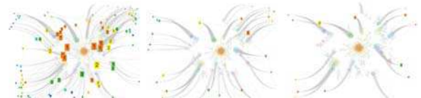
Figure 10: Lens: Lift the focused items up and keep others in the original view plane. (From left to right: threshold retweeting number is 5, 15, and 50, respectively)
