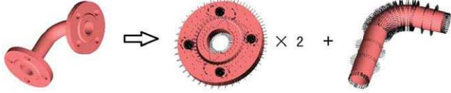
**Fig. 2.** The illustration of the decomposed parts from an assembly. The pipe fitting is composed of 2 flanges and 1 adapter. The black line segments indicate the normals of their corresponding faces. Note that the normals in each watertight mesh are compatible.
