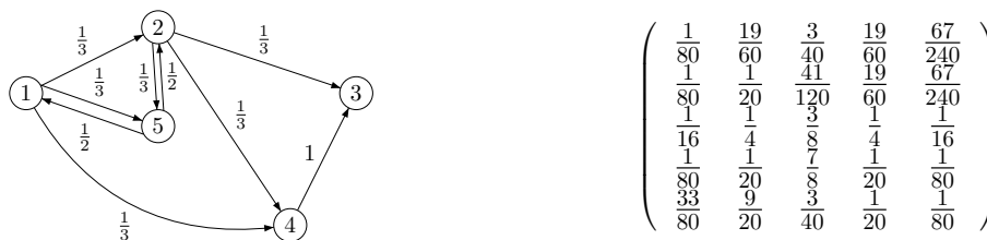
Fig. 3. (a) P , a Markov chain model of a subgraph of the World Wide Web and (b) the transformed irreducible and aperiodic chain P' in matrix form
