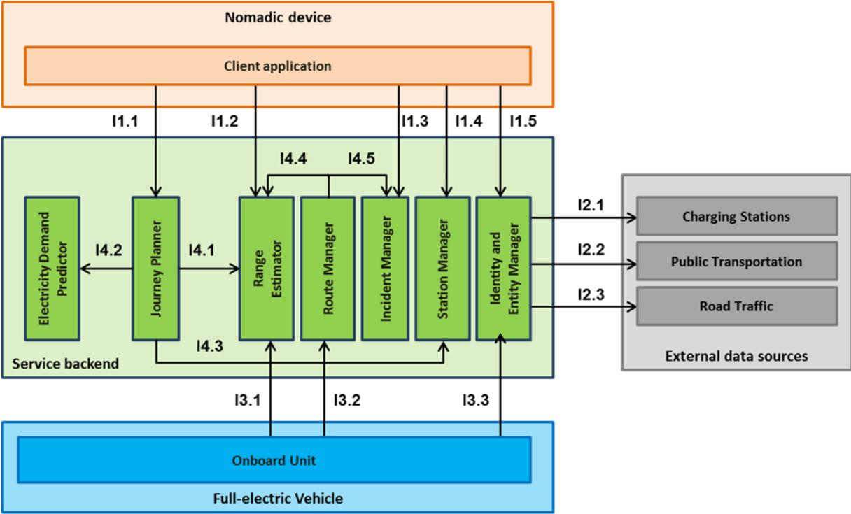
**Figure 1: high-level system architecture and required interfaces**
