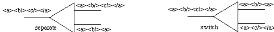
Figure 3 | Two custom dispatchers. The switch separates some elements from the others; this can be used for separating a bibliography with regard to the category of publications. The separator duplicates the input on the first output and sends specific elements on the others; this can be used for sending a book on the first channel, and its chapter and section titles on the other for building the table of contents.
