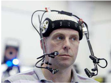
Figure 3 Head mounted camera system used to capture the facial expression of the actors.
