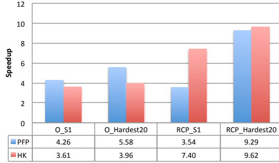
Fig. 5. Overall speedup of the proposed GPU algorithm w.r.t. PFP (left bars) and HK (right bars) algorithms.
