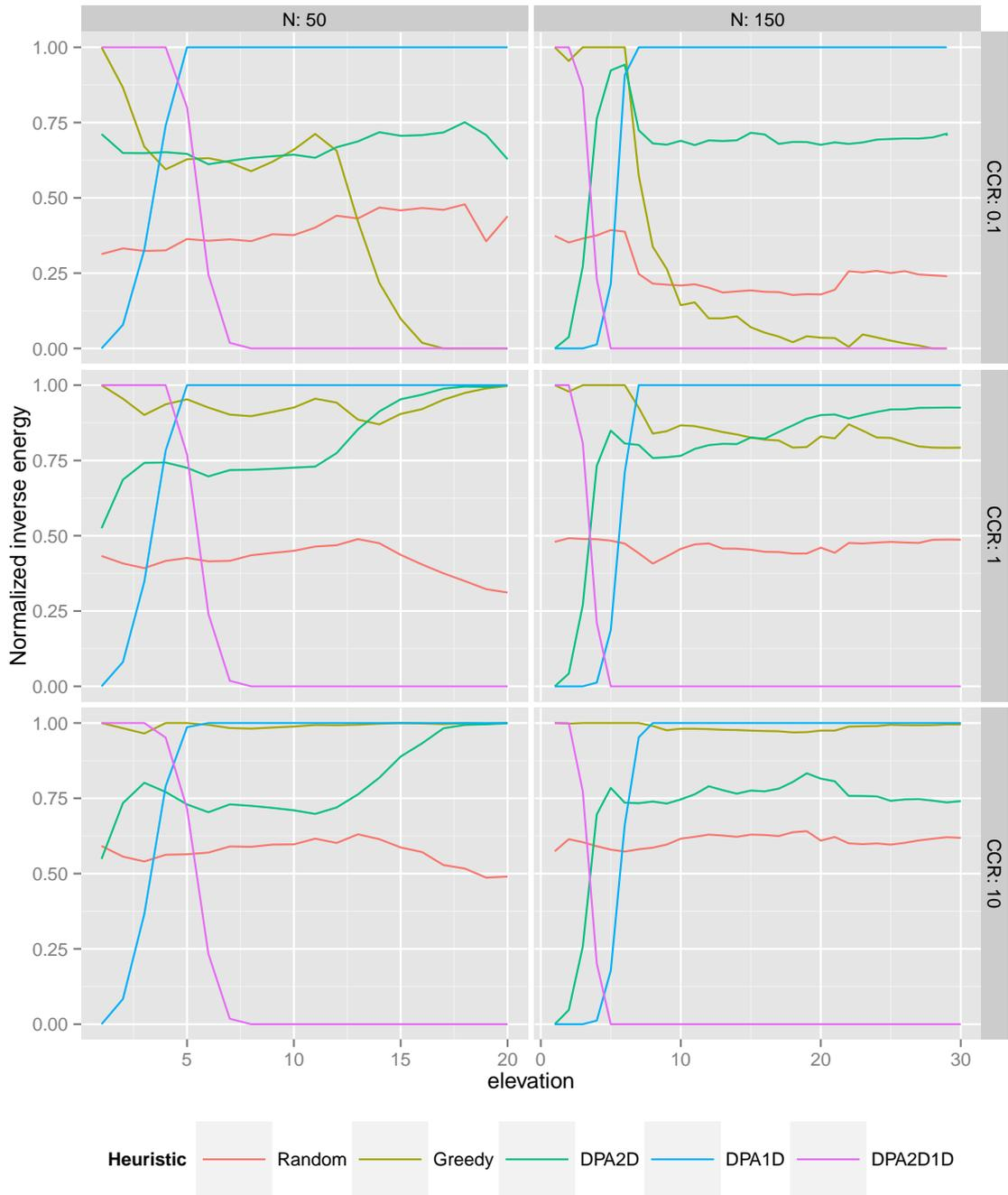
Figure 2. Normalized energy inverse on a random set of applications for a  $4 \times 4$  CMP grid.
