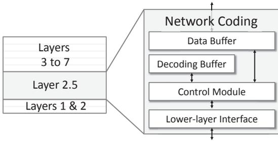
Fig. 3. Network Coding (NC) Layer - Decomposition
