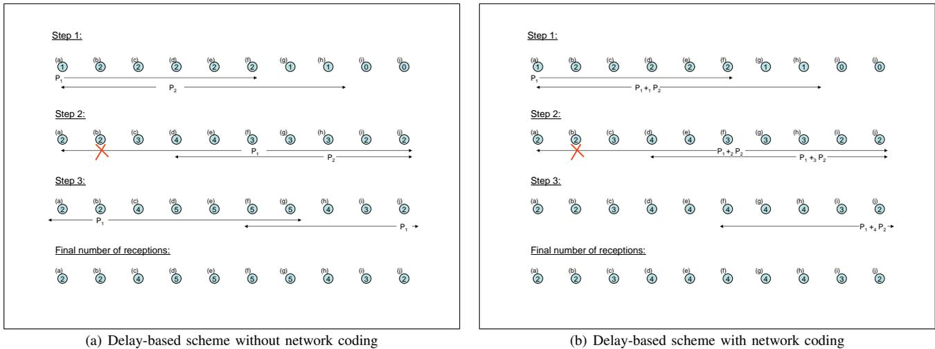
Fig. 4. An example of the dissemination of two messages with and without network coding. Node ‘a’ generates a packet  $P_1$  and node ‘d’ a packet  $P_2$ . The retransmission from ‘f’ is not received by ‘b’.
