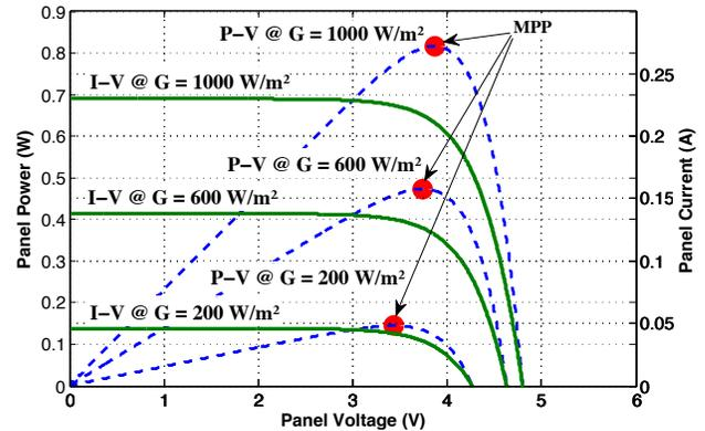
Fig. 5. PV panel current-voltage and power-voltage characteristic.
