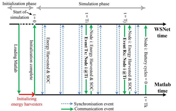
Fig. 2. Interactive co-simulation of WSN<sub>et</sub> and MATLAB.
