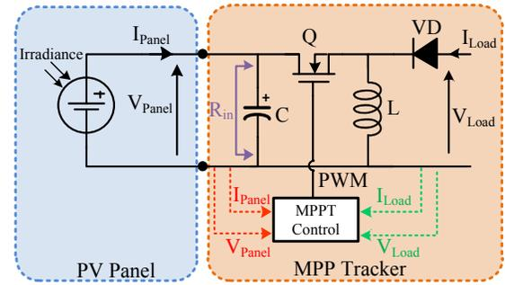
Fig. 4. Block diagram of solar energy harvesting system.
