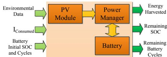
Fig. 3. Global architecture of the energy harvesting system.
