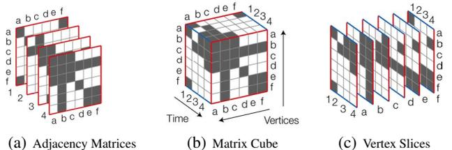
**Figure 1. The Matrix Cube.** (a) Each time step of the network (1,2,3,4), is represented as an adjacency matrix. (b) The Matrix Cube results from stacking those matrices. Red edges of the cube hold nodes and correspond to the rows and columns of the constituent adjacency matrices; blue edges of the cube hold time steps. (c) Slicing the cube along one of the vertex dimensions yields *vertex slices*.
