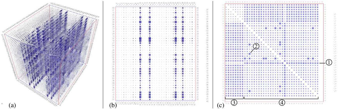
**Figure 9. ALMA dataset.** (a) Overview of RMS in which four time steps seem to stand out. (b) The vertex-projection view of RMS confirms this and provides additional detail. (c) The time-projection view on AMP, showing an abnormal behavior of one specific antenna ①, various baseline specific outliers such as ②. A different behavior of the first eight antennas compared to the other ones is clearly visible: ③ vs. ④.
