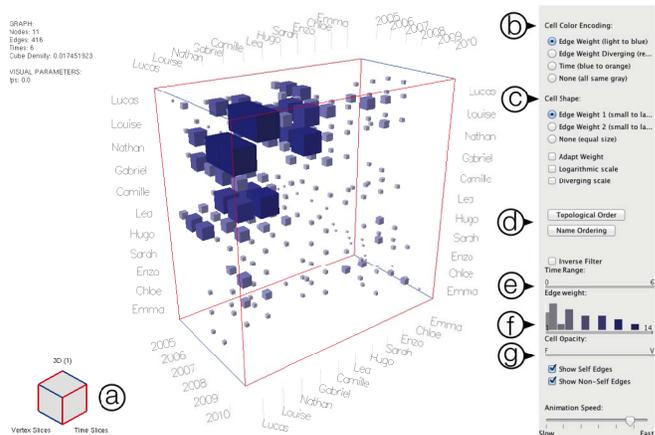
**Figure 2. Cubix UI screenshot.** a) Cubelet Widget, b) Cell color encoding, c) Cell shape encoding, d) Vertex ordering, e) Time range slider, f) Cell weight filter with histogram indicating edge weight distribution, g) Cell opacity.
